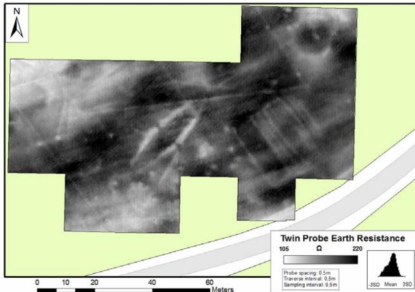
Figure 3: Twin probe Earth Resistance Survey from the summer of 2010 conducted by Arne Anderson Stamnes.
