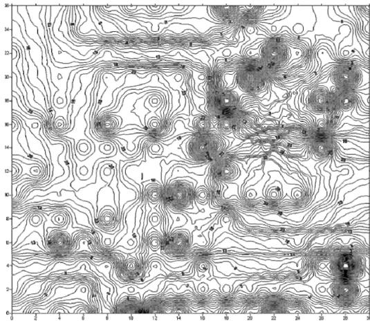
*Fig. 2 (above): Geomagnetic anomaly contour map of the total magnetic intensity field at the Yasilah archaeological site, northeastern Jordan.*
