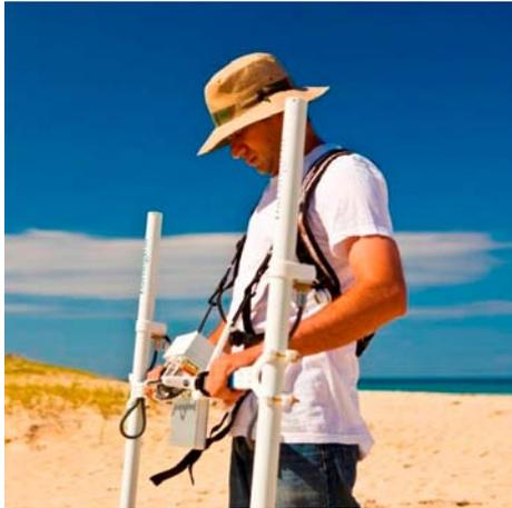
The Grad601 Gradiometer is an ideal instrument for magnetometry surveys in archaeology and for pipe and cable location. Since its introduction in 2004, it has rapidly gained an enviable reputation for its ease of use, automatic set-up and excellent stability. With a 1m vertical sensor separation, and a 0.03nT resolution, recorded data is of a very high quality, whilst fluxgate technology ensures the Grad601 is one of the lightest instruments available.
