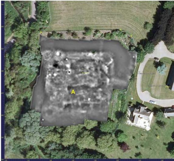
Figure 1: Northamptonshire Archaeology 2009 ground resistance survey result [1], highpass filtered. White represents resistance higher than the local mean (shown as grey), black lower.
