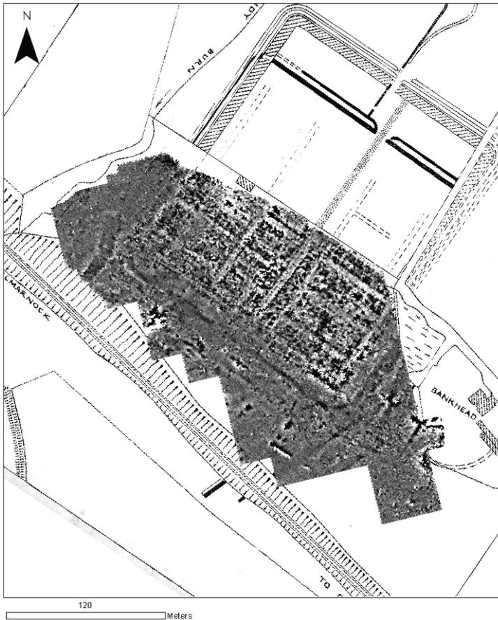
*Fig 1: Grey-scale graphic of the (Bartington) magnetic survey of the southern part of the fort at Dalswinton superimposed over the fort's plan. Black shows positive values.*
