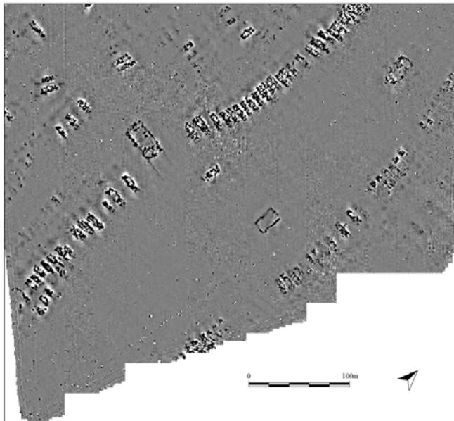
Figure 1: Nebelivka: geomagnetic survey (greyscale range: white - 15nT to black +15nT)
