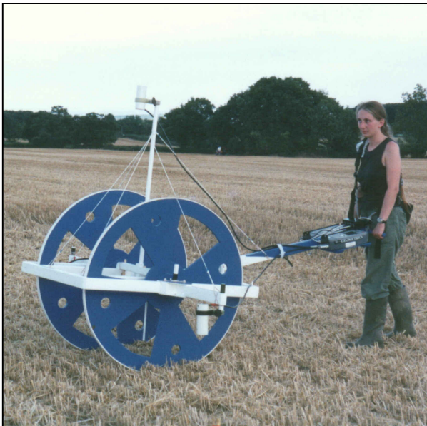
Fig. 1 Early "gradiometer", 3x 1m-spaced sensors
